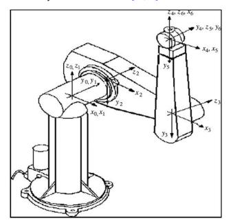
Figure 2. The PUMA 560 in the Zero Position with Attached coordinates Frames Shown [20]
