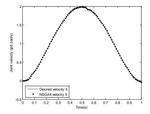
Figure 24. Desired and NSGAII joint velocities qp5
