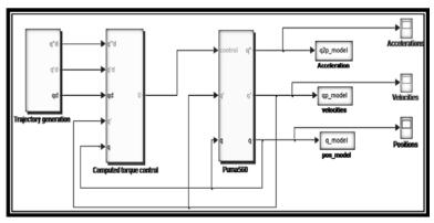
Figure 4. Simulink diagram of the simulation loop of the Puma 560 arm manipulator
