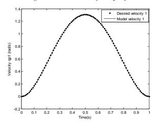
Figure 13. Desired and model joint velocity qp1
