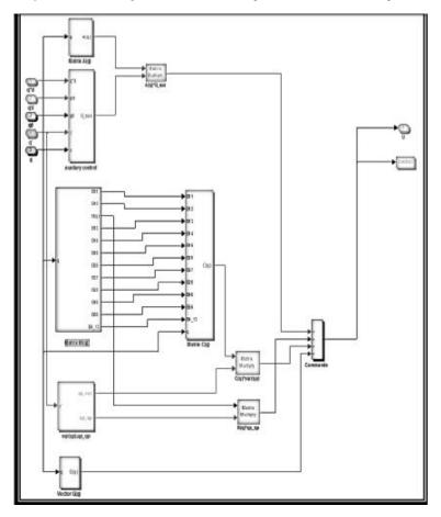
Figure 5. Simulink diagram of the computed torque control
