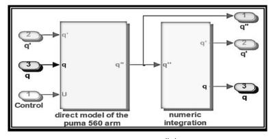
**Figure 6.** Block diagram for  $\ddot{q}, \dot{q}$  and q
