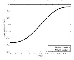
Figure 20. Desired and NSGAII joint angles q5
