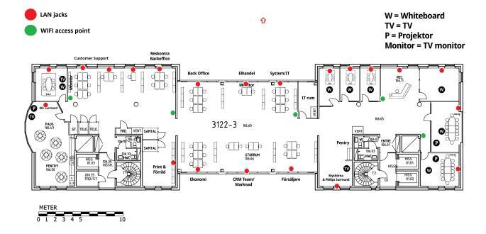
Figure 3: The new office with its APs and LAN jacks (i.e., RJ45 jacks).
