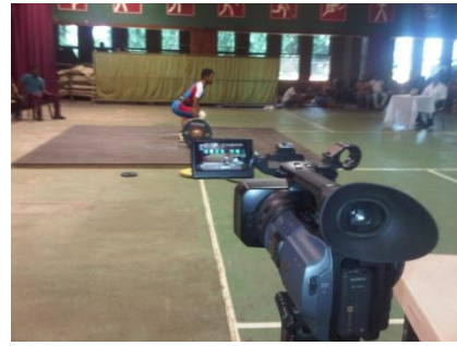
Figure 5-Capturing data in National Weightlifting Championships, Camera is perpendicular to bar motion.
