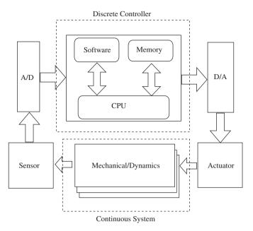
Fig. 1. Embedded system architecture.
