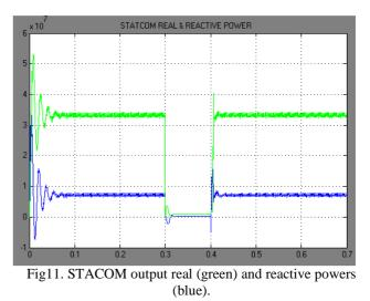
The system with STATCOM controller, a three phase to ground fault occurs between 0.3s to 0.4s are shown in figures 8 to 11. If comparing without and with STATCOM from Fig 6 and 8, the speed decreased to zero without STATCOM, but with STATCOM, the speed nearly maintained constant. From Fig 7 and 9, severe surge currents are produced at the starting of fault and clearance of fault without STATCOM, where as there are no surge currents produced with STATCOM.
