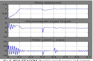
Case 3: with STACOM and with three phase to ground fault in the system
