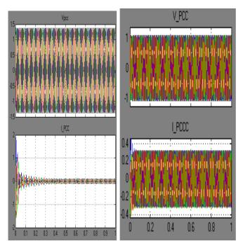
Fig 5. Without STACOM (left side) and with STACOM (right side) showing output voltage and current waveforms in pu
