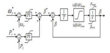
Fig. 1. Wind turbine pitch angle controller
