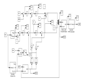
Fig. 2. Control scheme of the STATCOM.
