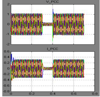
Fig9. With STACOM showing output voltage and current waveforms in pu with a 3PHG fault between 0.5 to 0.6s
