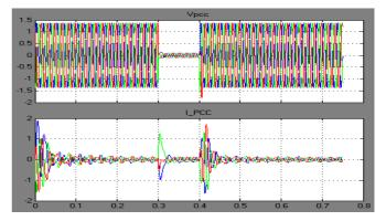
Fig7. Without STACOM showing output voltage and current waveforms in pu with a 3PHG fault between 0.5 to 0.6s
