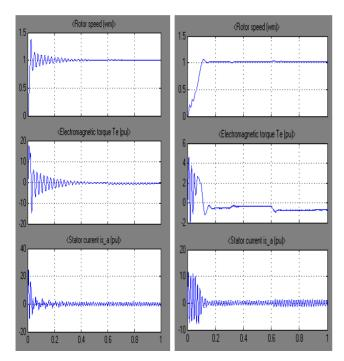
Fig 4. Without STACOM (left side) and with STACOM (right side) showing speed, torque and current waveforms in pu.
