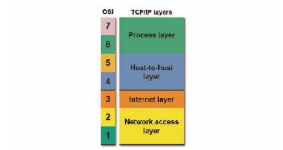
The OSI model describes computer networking in seven layers. While there have been implementations of networking protocol that use those seven layers, most networks today use TCP/IP. But, networking professionals continue to describe networking functions in relation to the OSI layer that performs those tasks. The TCP/IP model uses four layers to perform the functions of the seven-layer OSI model.
