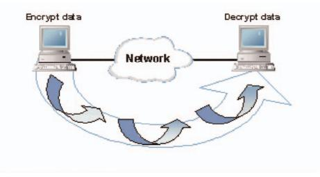
Layer 6, the presentation layer, is responsible for how an application formats the data to be sent out onto the network. The presentation layer basically allows an application to read (or understand) the message. Examples of presentation layer functionality include:
