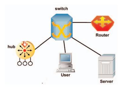
Some of the layers use equipment to support the identified functions. Hub related activity is "Layer One". The naming of some devices designates the functional layer such as "Layer Two Switch" or "Layer Three Switch". Router functions focus on "Layer Three". User workstations and servers are often identified with "Layer Seven".
