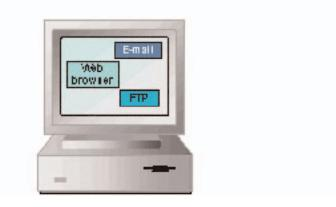
Layer 7, the application layer, provides an interface for the end user operating a device connected to a network. This layer is what the user sees, in terms of loading an application (such as Web browser or e-mail); that is, this application layer is the data the user views while using these applications.
