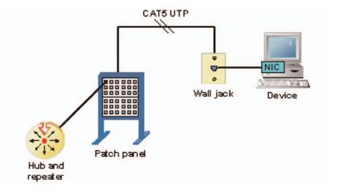
The physical layer of the OSI model defines connector and interface specifications, as well as the medium (cable) requirements. Electrical, mechanical, functional, and procedural specifications are provided for sending a bit stream on a computer network.
