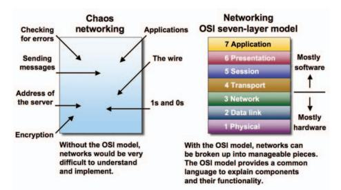
A networking model offers a generic means to separate computer networking functions into multiple layers. Each of these layers relies on the layers below it to provide supporting capabilities and performs support to the layers above it. Such a model of layered functionality is also called a "protocol stack" or "protocol suite".
