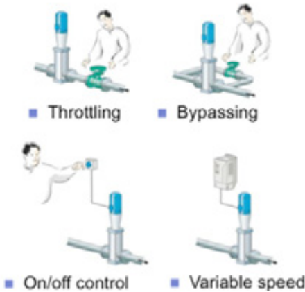
Figure 2.7 - Common flow control methods, (ABB Oy) Drives, 2006)
