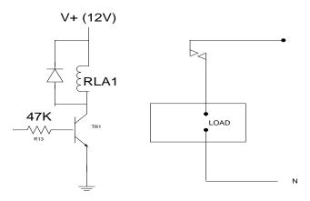
Figure 5. Schematic diagram of a transistor switching with relay
