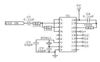
Figure 3. Circuit diagram of DTMF decoder
