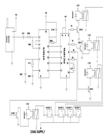
Figure 8. Comprehensive circuit diagram of the system
