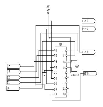
Figure 4. Circuit diagram of microcontroller section
