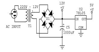
Figure 7. Power soupply stage
