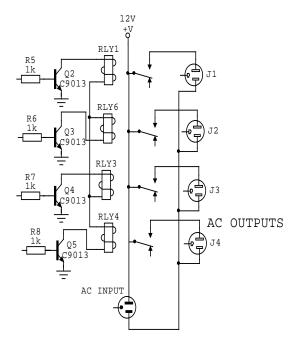
Figure 6. Circuit Diagram of the Switching Stage
