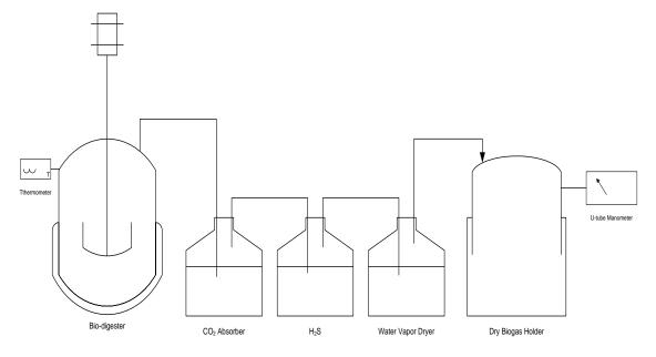
Figure 1. Flow diagram of the biogas production unit
