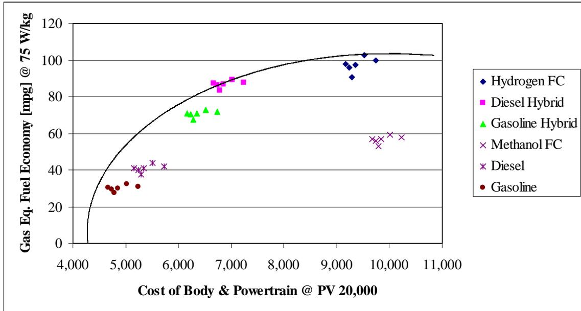
Figure 23: Gasoline equivalent fuel economy and cost of vehicle production (body PV 20,000 and propulsion system cost estimation) for a vehicle performance of 75 W/kg
