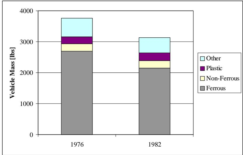
Figure 2: Passenger Car Material Content (OTA, 1995)
