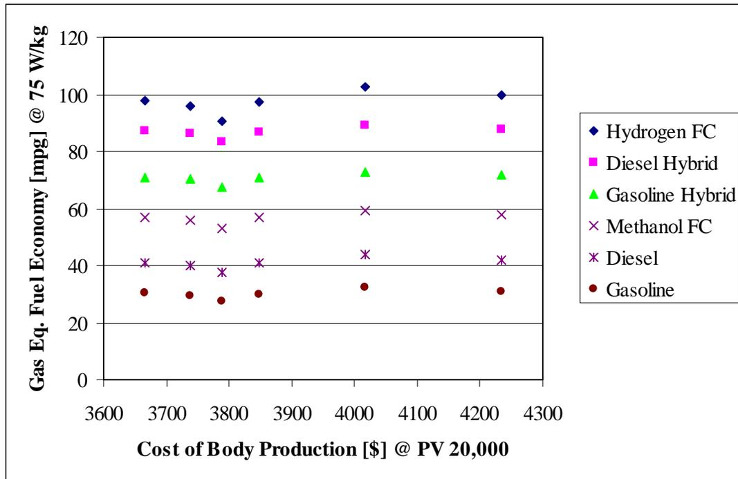
Figure 22 Gasoline equivalent fuel economy and cost of body production at production volume of 20,000 and a vehicle performance of 75 W/kg for all propulsion technologies
