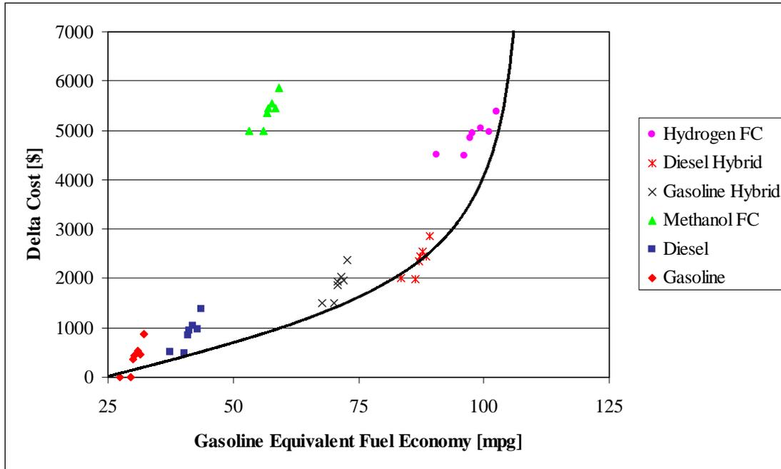
Figure 25: Vehicle cost (@ PV 125,000) with increase of gasoline equivalent fuel economy (Baseline of delta cost: steel unibody gasoline powered vehicle)
