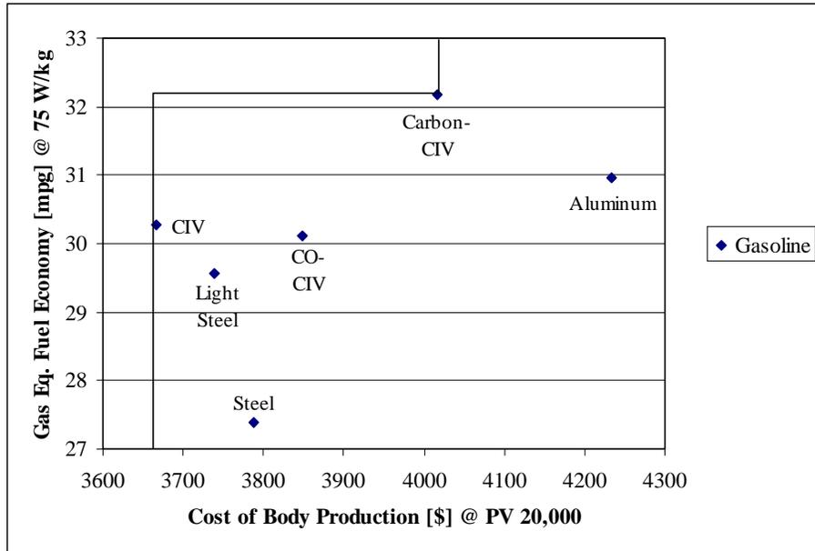
Figure 20: Gasoline equivalent fuel economy and cost of body production at production volume of 20,000 and a vehicle performance of 75 W/kg for gasoline engines
