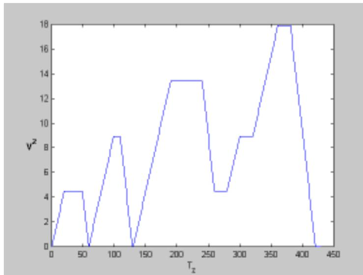
Figure 7: Urban cycle (simplified driving cycle)
