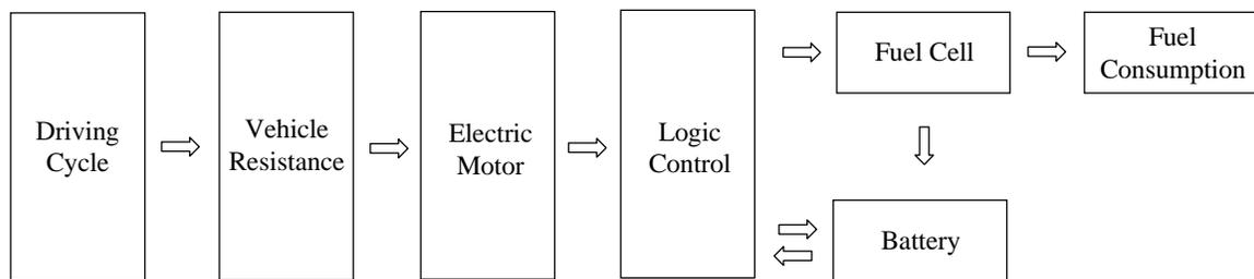
Figure 16: Calculation Logic for Fuel Cell Drivetrain
