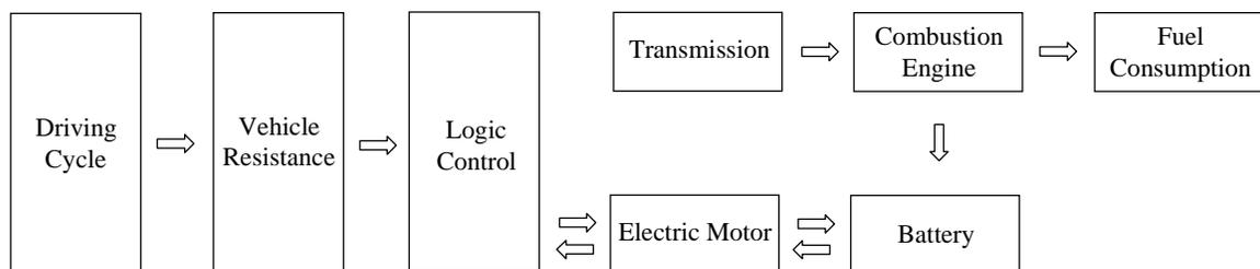
Figure 15: Calculation Logic for Internal Combustion Engines – Battery Parallel Drivetrain
