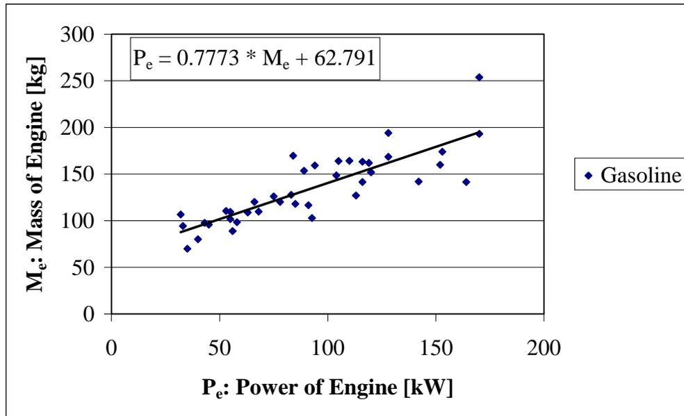
Figure 5: Power density of gasoline engines
