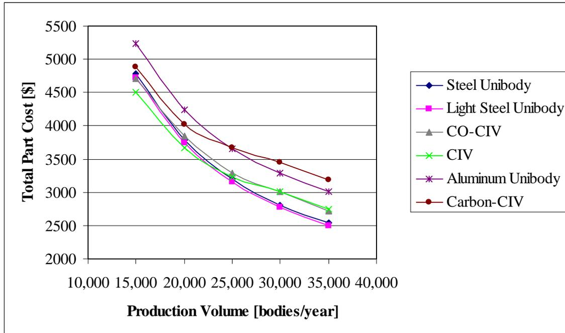
Figure 18: Total Production Cost of body designs at production volume 15,000 to 35,000
