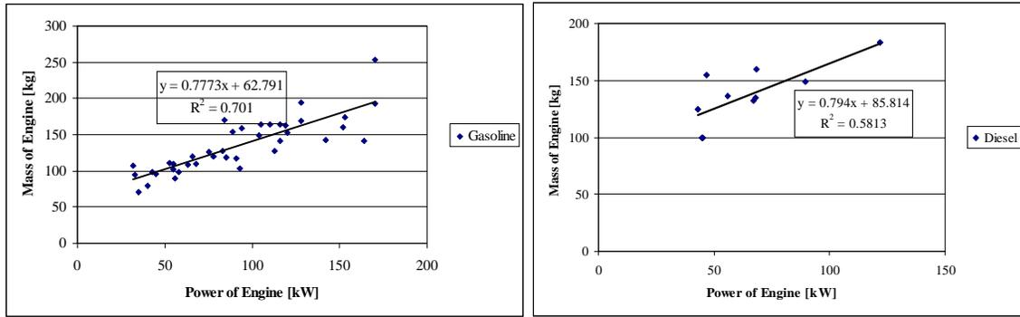
Figure 9: Mass to power correlation for gasoline and diesel engines
