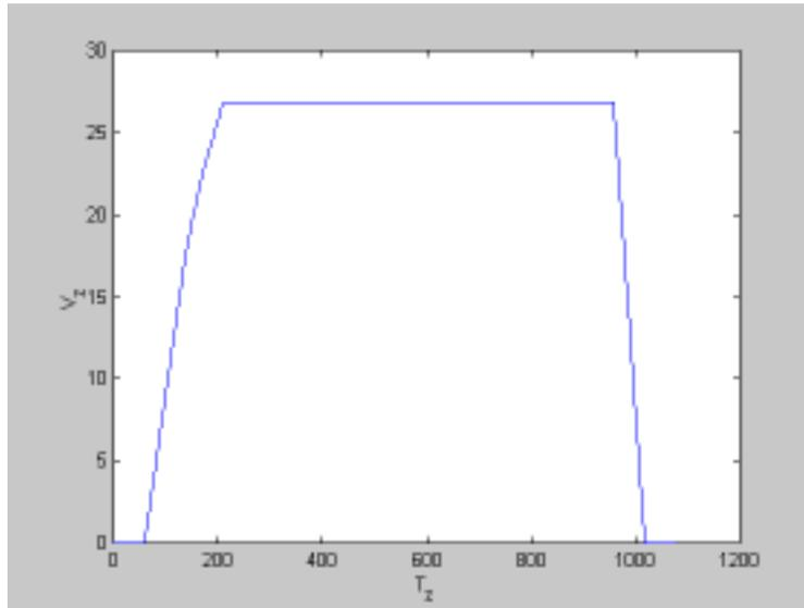
Figure 6: Highway cycle (very simplified driving cycle with one acceleration and one deceleration)
