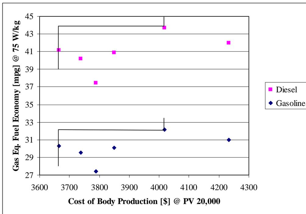
Figure 21: Gasoline equivalent fuel economy and cost of body production at production volume of 20,000 and a vehicle performance of 75 W/kg for gasoline and diesel engines
