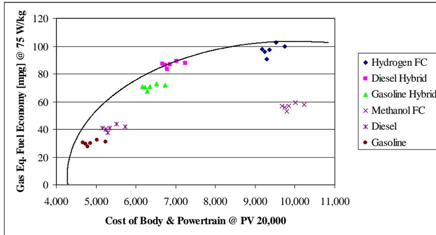
Figure 26: Gasoline equivalent fuel economy and cost of vehicle production (body PV 20,000; vehicle performance: 75 W/kg)
