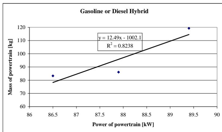
Figure 11 Mass to power correlation for gasoline or diesel hybrid engines
