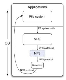
Figure 2.4. User-level file systems via kernel proxy.
