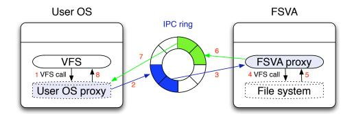
Figure 4.1. This figure illustrates the sequence of operations and data movement for handling a user OS VFS operation. The red numerals indicate the sequence. Note that data operations (e.g., read) require more steps in order to share memory between VMs.
