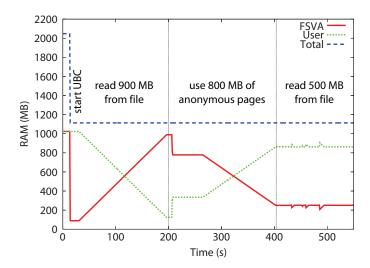
Figure 6.5. Unified buffer cache demonstration. This figures shows the amount of memory consumed by the user and FSVA VMs. As applications shift their memory access pattern between file system and virtual memory usage, the unified buffer cache dynamically allocates memory among the two VMs while maintaining a constant total memory allocation.
