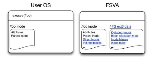
Figure 4.2. Metadata is duplicated between the user OS and FSVA OS, to maintain user OS functionality. The user OS proxy creates generic metadata structures in the user OS. File system-specific metadata, shown underlined for a Linux ext3 file system example, is only kept in the FSVA OS.
