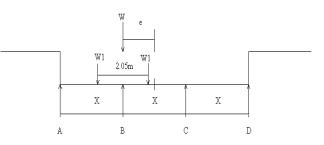
Fig. 3 Transverse Disposition of IRC Class AA Tracked vehicle
