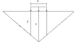
Fig. 6 Influence line for bending moment in girder Where:
