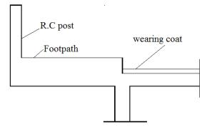
Fig. 4 Details of footpath, parapet and deck slab
