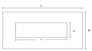
Fig. 2: Position of IRC Class AA Wheel Load for Maximum Bending Moment
