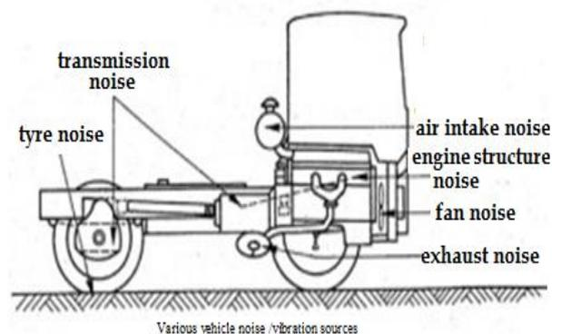
Fig. 5(b): Various vehicle noise /vibration sources
