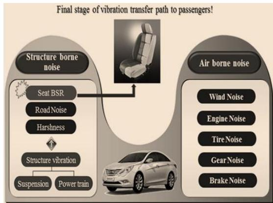
Fig.4 .vibration transfer path
