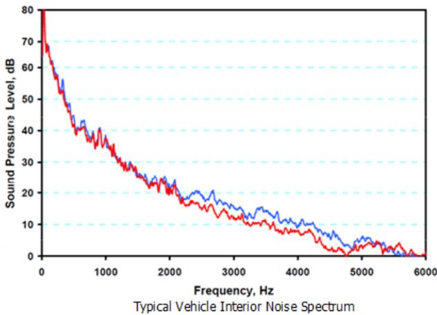
Fig. 6 . Typical Vehicle Interior Noise Spectrum
