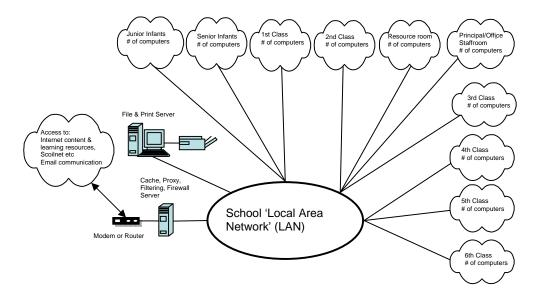
Fig 9: Typical Network Model for a Special school.
