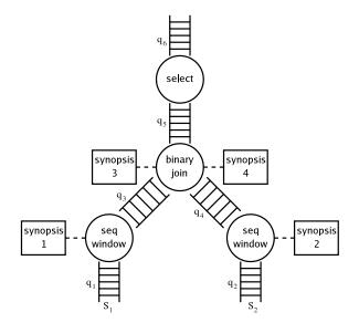
Fig. 2. A simple query plan illustrating operators, queues, and synopses.
