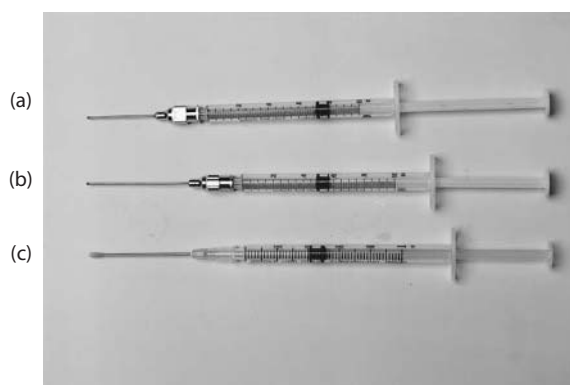
Figure 32.8 Syringes with a gavage needle. (a) 1.0 ml syringe with a 22 G \times 1.0 in. feeding needle; (b) 1.0 ml syringe with a 20 G \times 1½ in. feeding needle; (c) 1.0 ml syringe with a 20 G \times 1½ in. disposable feeding needle.
