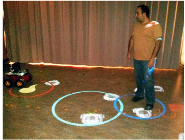
Figure 2. A person and a Pioneer 2AT collaborating on the herding task. The light bulb, pen, and lock are used to play the game. Circles are drawn around the robot and the person (red and blue, respectively).
