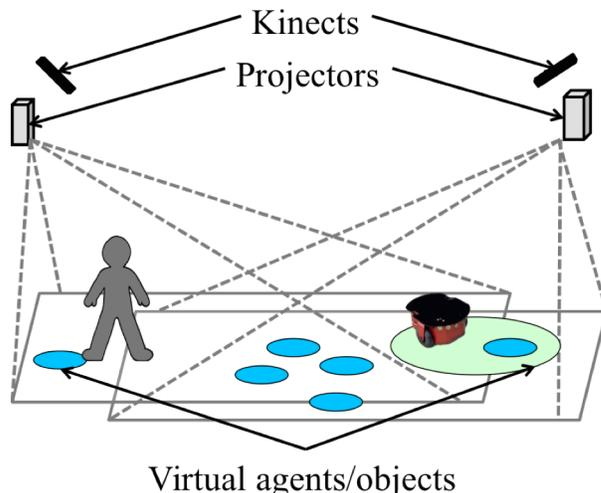
**Figure 1. A diagram of the experimental setup. Calibrated overhead projectors overlap to minimize shadowing. The task simulation uses person and robot tracking data from multiple Microsoft Kinects mounted near the ceiling.**
