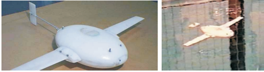
Figure 1.1: Experimental, laboratory-scale underwater glider ROGUE.
