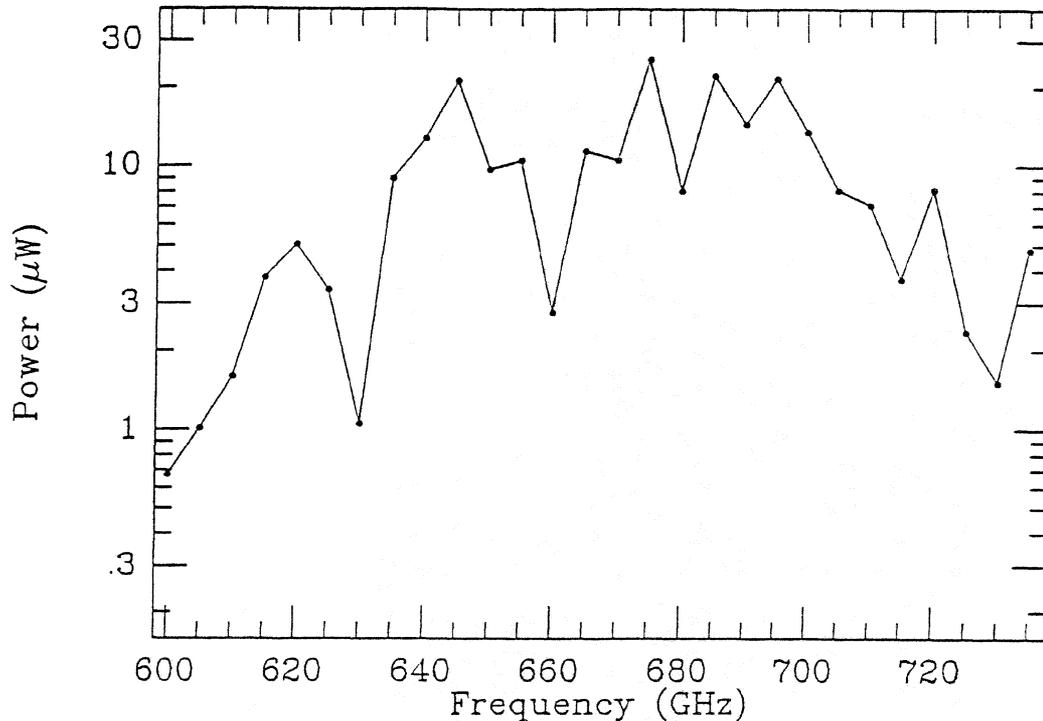
Figure 2: Output power as a function of frequency from the 600-720 GHz source.
