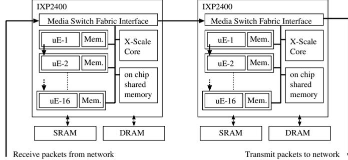
**Fig. 1.** Simplified diagram of IXDP2400 NP evaluation board
