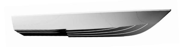
Fig. 1.4 Delta 29 SW with a Transverse Step
