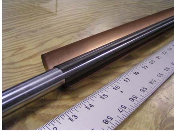
**Figure 3: Cured curved lamina mandrel and caul plate.**
