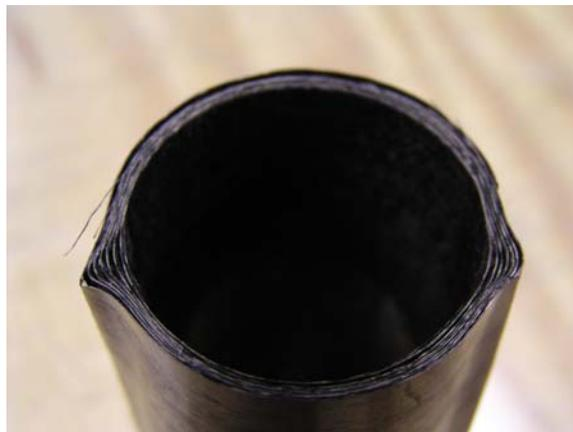
**Figure 5: Crimped coiled lamina as a result of autoclave and vacuum bag pressures.**
