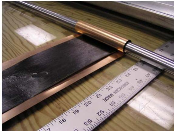
**Figure 4: Coiled lamina mandrel and caul plate.**
