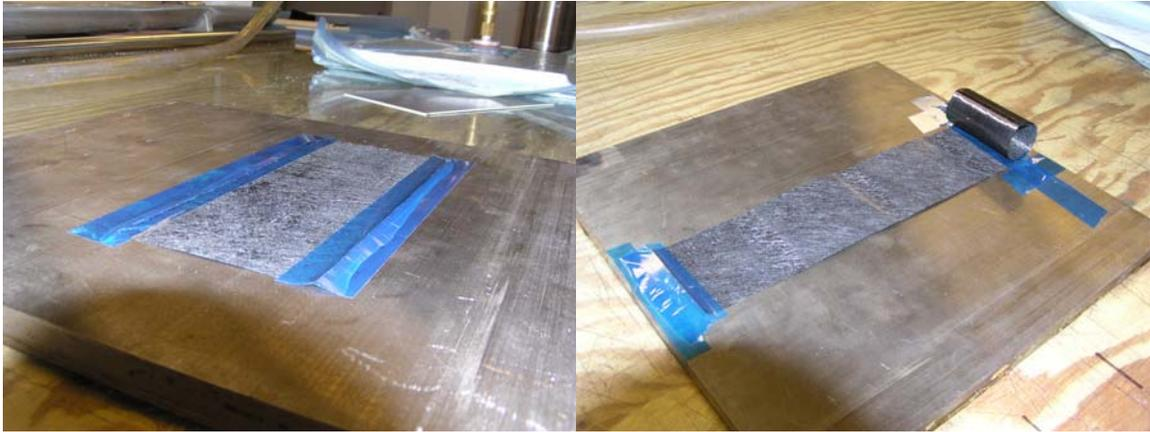
**Figure 6: Coiled and curved laminas taped to caul plates in preparation for bonding.**
