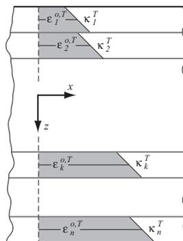
**Figure 7: Specification of pre-strains in an arbitrary laminate.**
