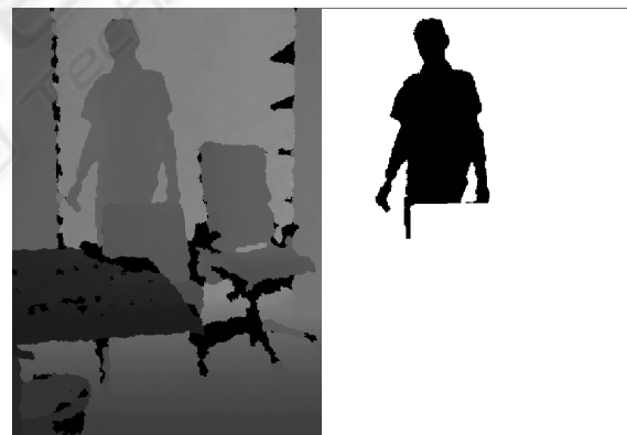
Figure 1: Foreground objects (right) are detected in depth images (left) taken by a static depth camera.
