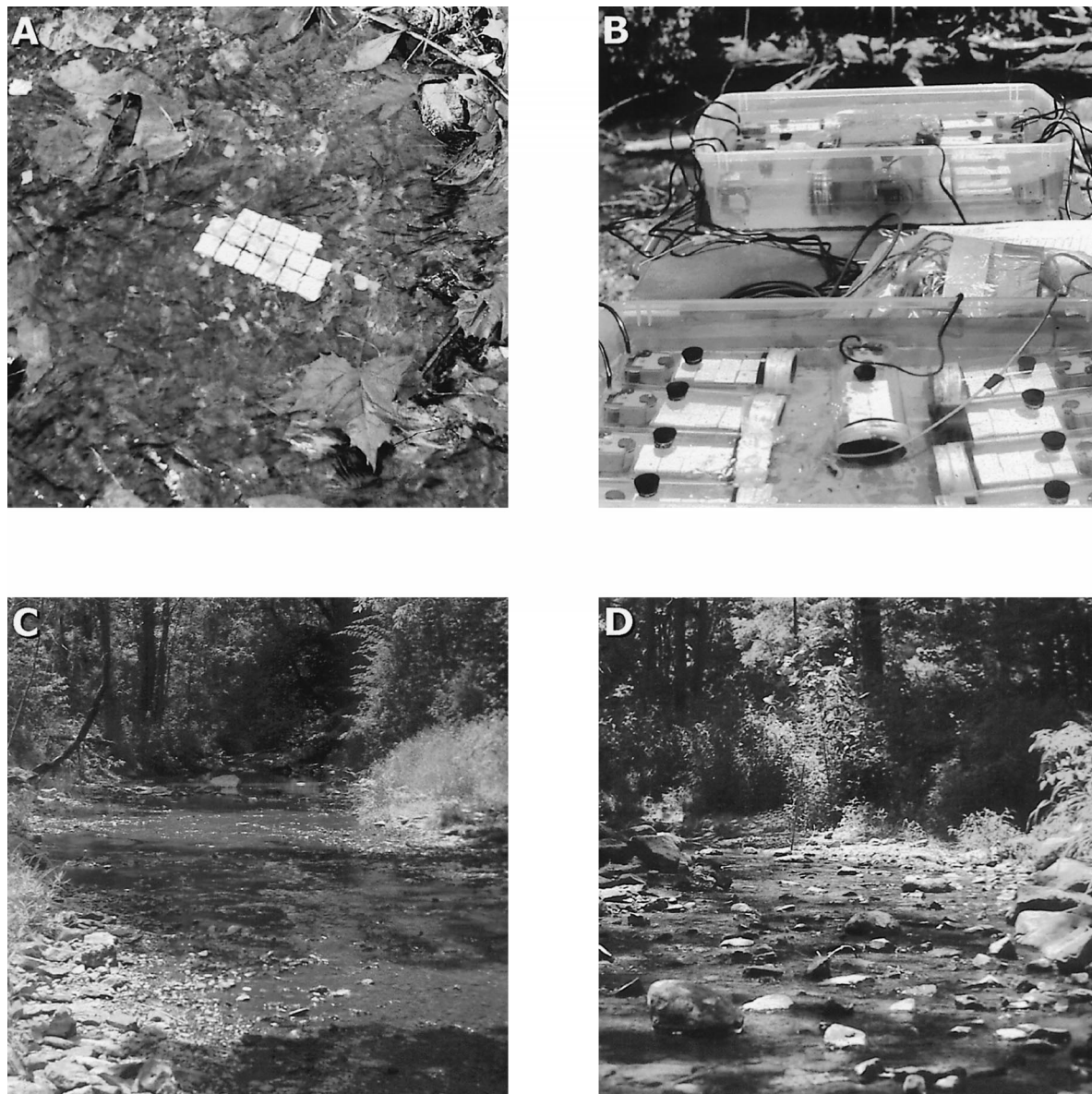
FIG. 1. (A) One of ten tile units that were placed on the benthic habitat of a low heterogeneity riffle. (B) The central incubation site showing tiles sealed inside 0.5-L metabolism chambers being held at a constant temperature in water baths. Also shown are examples of (C) low heterogeneity (LH) and (D) high heterogeneity (HH) riffles after manipulation of substrate variability.
