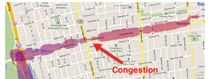
Fig. 5. Velocity plotted with varying line width instead of color-coding
