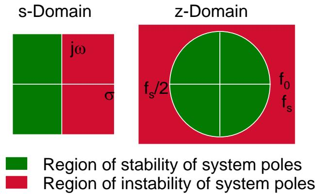
Stable systems have their poles (feedback elements) located in the left hand half of the s-plane and these are mapped to a region that lies within the “unit-circle” of the z-domain. Zeros (feedforward elements) can lie anywhere on either plane.
