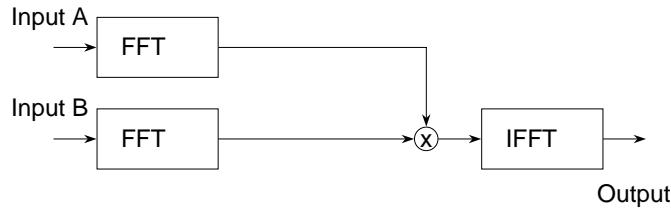
The FFT of a system (e.g. a filter) impulse response is the transfer function, the finite length transfer function is applied to an “infinite length” signal so an overlap method will be required (E.G. Overlap and add). It is important to use the correct coefficients E.G. for a low-pass filter can not just set high frequency coefficients to zero as this generates a time domain  $\sin(x)/x$  function.
