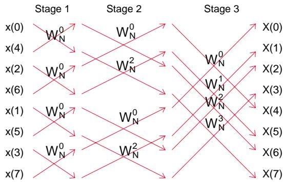
With the forward and inverse transforms, either the input or output data sets must be in a non-linear format that uses a bit reversed address style. Most modern DSPs are able to handle this directly in hardware so converting the data back into a linear order often requires no overhead to the operation.
