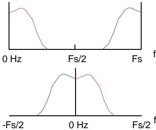
The first format is often used in baseband applications e.g. speech and system analysis, where as the second is more common in H.F. communication applications, where  $f_c$  is is hetrodyned down to D.C. The results are no different but sometimes make post processing easier.
