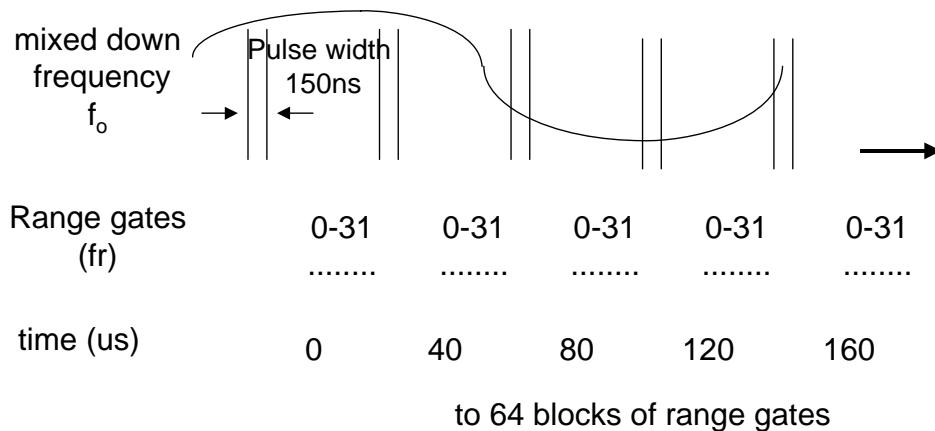
Each range gate corresponds to a number of cycles at the transmitted frequency, as shown below.
