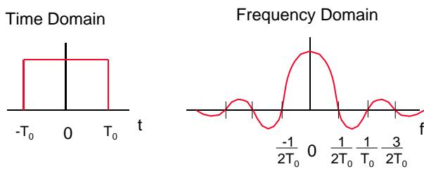
Looking at the effects from a different perspective we see the *edge effect* more clearly. Using this approach we can also see how to remove the edge effect by using a window that tapers to zero at the extremities.
