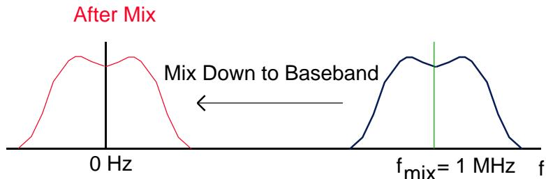
Typical applications of the zoom-FFT include; ultrasonic blood flow analysis, R.F. communications, mechanical stress analysis and Doppler radar.
