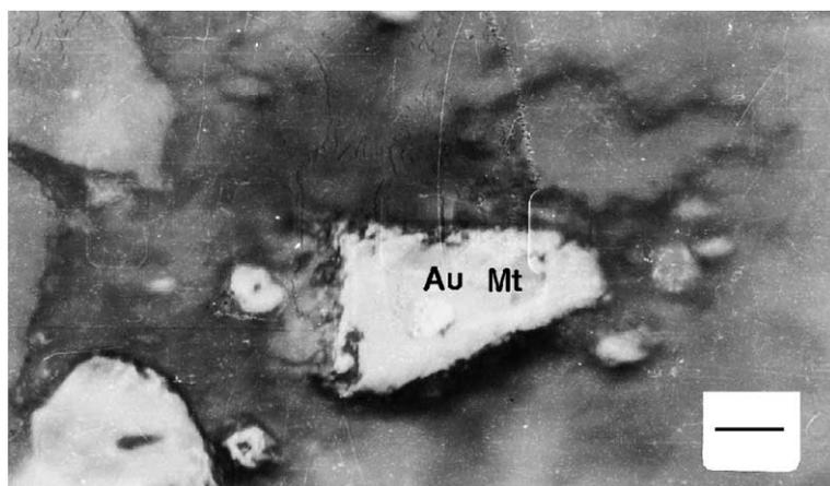
Fig. 13. Photomicrograph showing gold speck (Au) hosted in magnetite (Mt) host, Um Monqul gold prospect, Eastern Desert, Egypt. Reflected light, bar length represents 0.05 mm (from Botros and Wetait, 1997).
