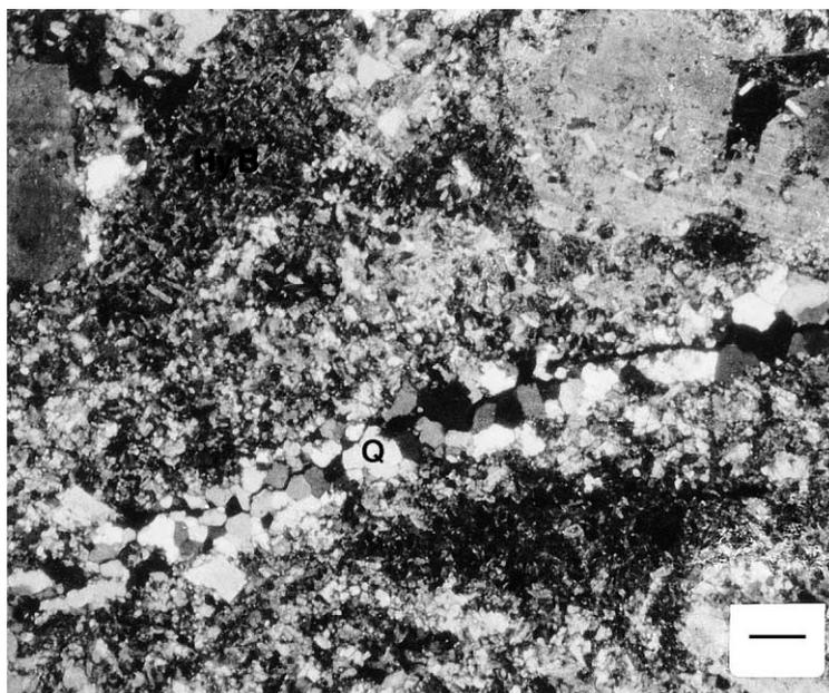
Fig. 12. Photomicrograph shows a clustering of hydrothermal biotite (Hy.B) in the form of a biotite crystal in rhyodacite porphyry. Notice the presence of secondary quartz veinlet (Q). Plane polarized light, crossed nicols, bar length represents 1.22 mm (from Botros and Wetait, 1997).
