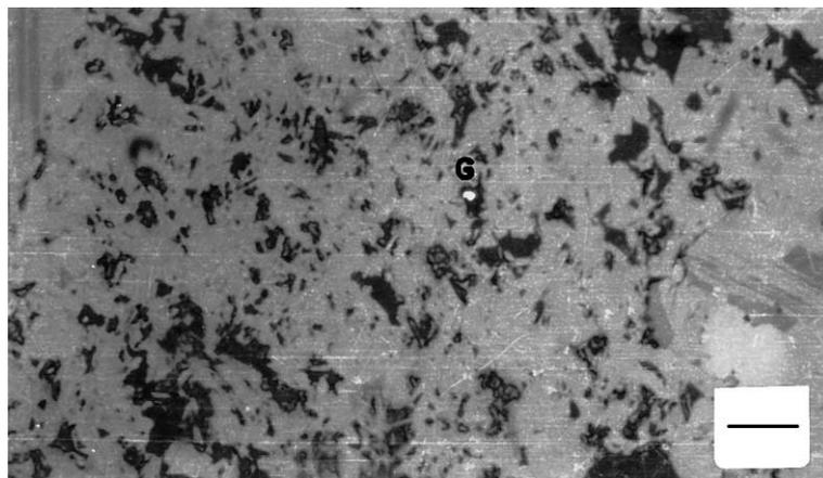
Fig. 10. Photomicrograph of Algoma-type (BIF) showing minute gold speck (G) enclosed in the gangue minerals, Abu Marawat gold prospect, Eastern Desert of Egypt. Bar length represents 0.02 mm. (from Botros, 1991).
