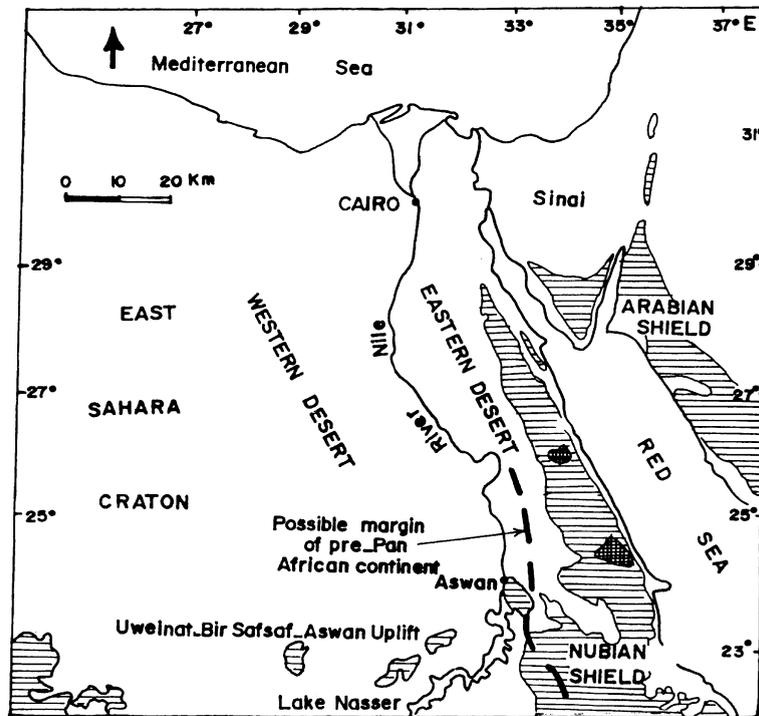
Fig. 3. The possible boundary between the East Sahara Craton and the rocks of the Panafrican belt and the tectonic windows (compiled from El Gaby et al., 1988; Greiling et al., 1994). ▨ Rocks of the Panafrican belt, ▩ Windows.
