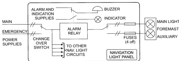
Figure 3.16: Navigation lights circuit.
