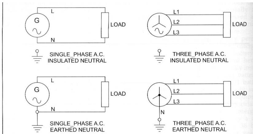
Figure 1.1: Insulated and earthed neutral systems.
