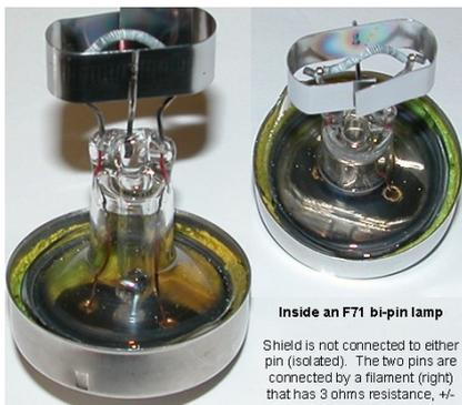
Figure 3.4: A fluorescent lamps filament.
