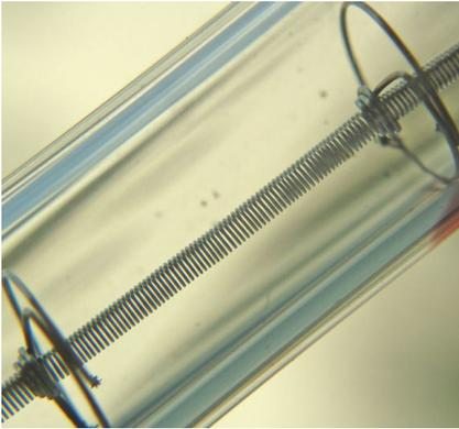
Figure 3.2: Tungsten-halogen lamp.
