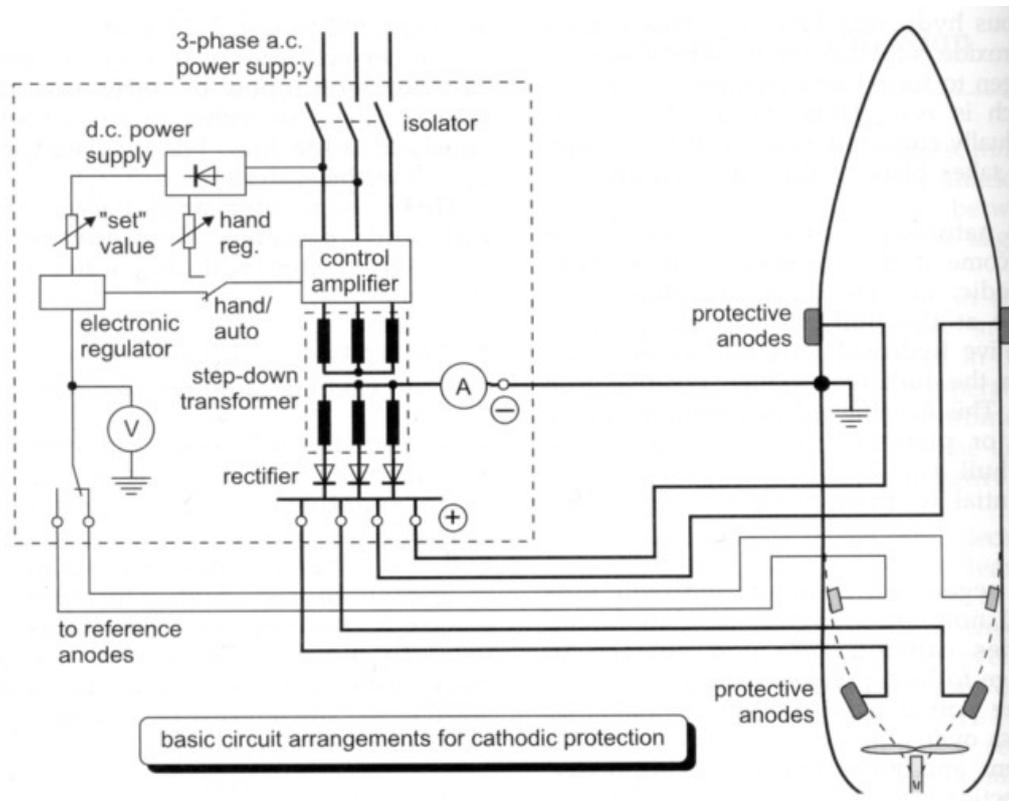
Figure 3.25: Ships anodes and impressed current control system.
