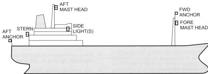
Figure 3.15: Ship's navigation lights arrangement.
