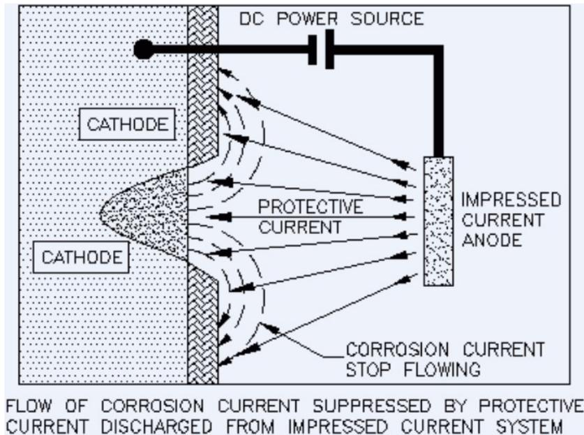
Figure 3.24: Impressed current system.
