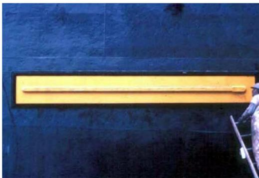
Typical Hull Mounted ICCP Anode - Primary Dielectric Shield (Courtesy Deepwater)
