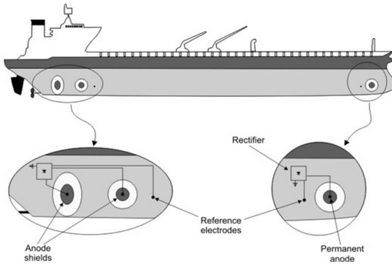
Figure 3.26: Impressed current system on a tanker.
