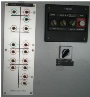
Figure 3.18: Signal lights switchboard.
