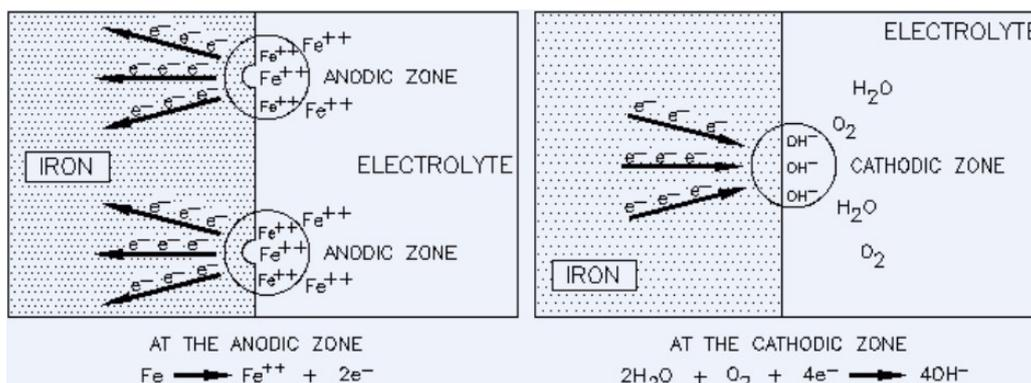
Figure 3.19: anodic reaction and cathodic reaction.
