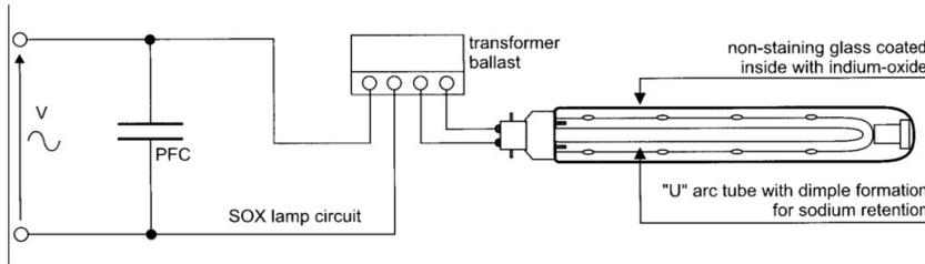
Figure 3.11: SOX lamp and circuit.
