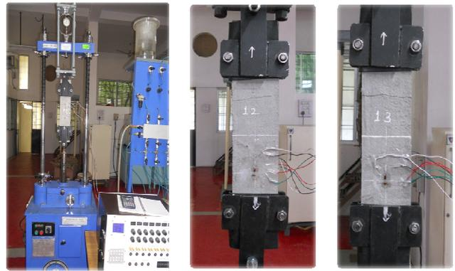
Fig. 3 Tensile Test Set – up with Test Specimens
