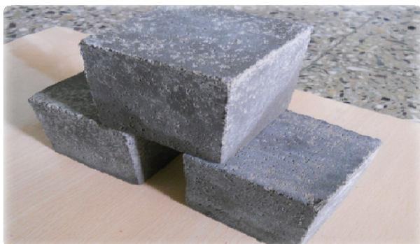
Fig. 2 Cube Specimen for Compressive Strength
