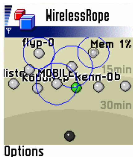
Figure 1. A screenshot of the Wireless Rope J2ME software. The black circle represents the owner, while devices in the environment are classified as familiar (green) or strangers (grey). Devices move closer to the black circle as they spend more time within range.
