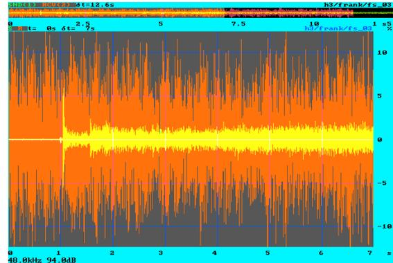
Fig. 1: Convergence behavior of a background noise reduction algorithm: dark (red) original signal: car noise in a constant driving condition (130 km/h), light (yellow) processed (output) signal
