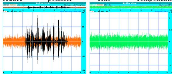
Fig. 4: Left - background noise signal (red/dark gray) and far end speech signal (black); right - transmitted background noise signal
