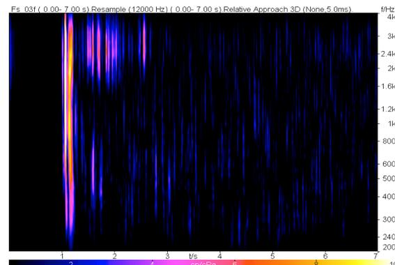
Fig. 3: "Relative Approach" analysis of the processed (output) signal; bright colors indicate audible components in time or frequency
