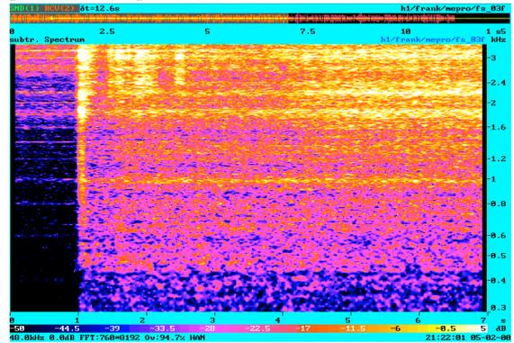
Fig. 2: Spectral difference between processed (output) signal and original (background noise) signal; bright colors = high differences, dark colors = low differences
