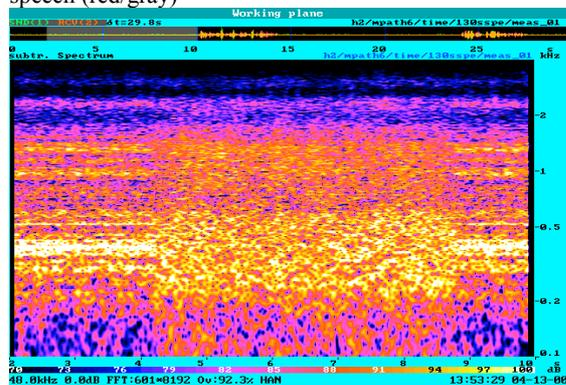
Fig. 6: Spectral difference between transmitted background noise signal and original background noise
